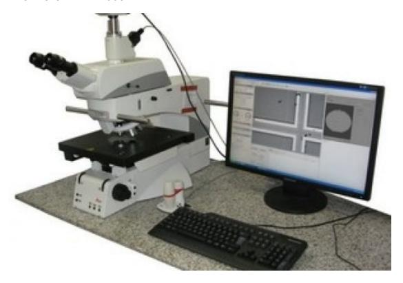
Universal semiconductor microscope with option for layer thickness measurement.
