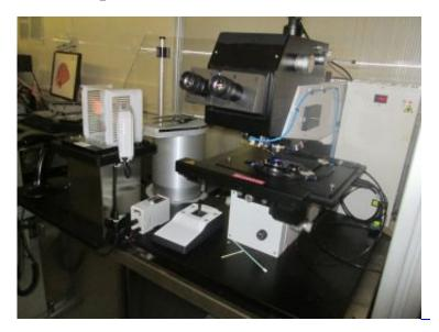
**Inspection** of masks used to produce wafers.
