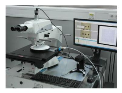
Configuration of the Leica DM8000 by using the Promicron MCS software for semi-automatic wafer amd MEMS Inspection.
