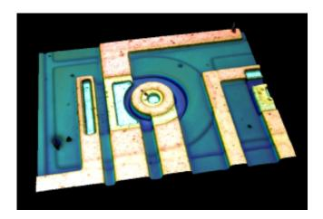
MCS Confocal - software for 3D metrology in the nanometer range with a light microscope:
