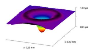
In contrast to interferometry, where vertical resolution is independent of the magnification, confocal discrimination increases sharply with the numerical aperture (NA) of the lens used.
