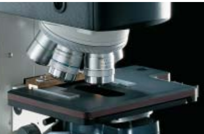
Industry stage , travel distance 76 x 50 mm, 110° rotation, with industrial slide holder
