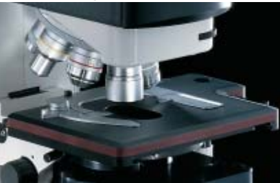
Bio I stage , travel distance 76 x 25 mm, 110° rotation, with single-hand slide holder
